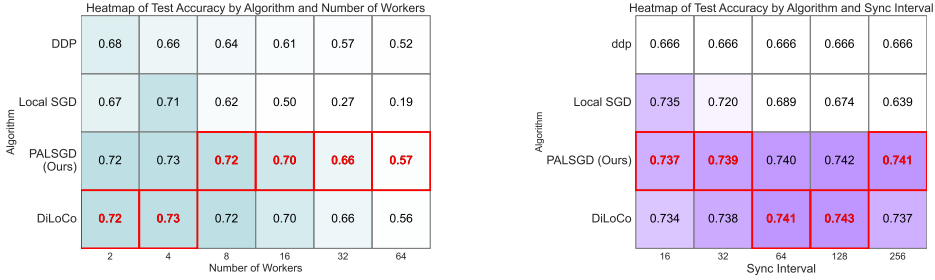
Figure 1: Simulation Experiments: (Left) Comparison of K (Number of workers) with H=32. (Left) Comparison of H (Sync Interval) with K=4. PALSGD has low sensitivity to K and H, and achieves high accuracy consistently.
